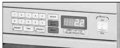
Crosslinker Control Panel
